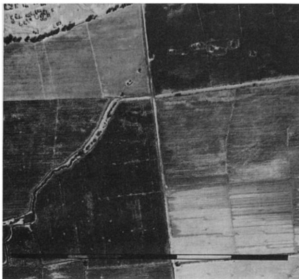
Figure 8. Aerial photograph of La Gobernadora taken in March 1970. The lower end of the puquio is open trench ending at a small kocha , visible near the lower left corner of the photograph. The middle section of the puquio is filled-trench gallery; portions have caved in and been left as open trench. The upper section of the puquio is tunneled gallery. Traces of an abandoned second branch can be seen just below the path that forms the field line running east-west to the right of the puquio.
